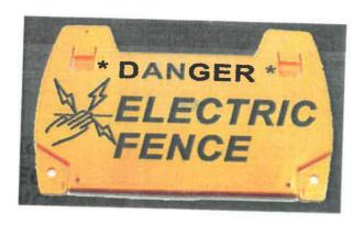
Warning signs must be placed along the fence line to warn of the existence of an electrified fence. These must be placed at 10m intervals along the fence, at gate ways or whenever there is a change of direction. Wire clips on the warning sign reduce installation time.
